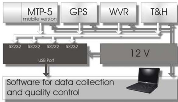
Fig.1 The schema of the mobile system where MTP-5 - meteorological temperature profiler, WVR - water vapor radiometer, T&H - temperature and humidity sensor.
